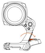
To adjust the correct tension of the base onto the M1913 rail, the QD Lever must be in the absolute down/ open position. Squeeze the spring tensioned base and rotate the nut clockwise to tension or counter clockwise to loosen.
