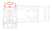
Place the magnifier in the desired location on your M1913 Rail. Ensure you seat the side of the base without the QD Lever first. Pull the QD Lever up into the closed position until you feel it snap.
