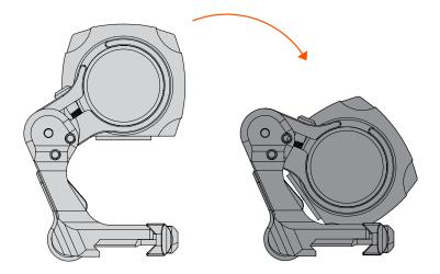
Bring the magnifier into the up position. From the inside of the base, depress the safety on the interior of the integrated FAST<sup>TH</sup> OD Lever. Push outward and the OD Lever will open fully. The OD Lever may need to be held flush with the mount base while depressing the safety.
