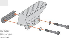
Place the FAST<sup>TM</sup> Absolute Riser on the M1913 Rail in desired location. If using the included Rail Clamp, move to step 2. If using the optional FAST<sup>TM</sup> QD Lever (sold separately), jump to step 3.
