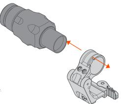
The FAST™ FTC 30mm mount uses a force-to-overcome mechanism. Grasp the magnifier body and pivot assembly down to the stowed position. Repeat in reverse to bring the magnifier back into the active position.
